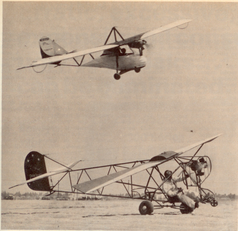
Cycloplane flight trainer passing over a two-seat ground trainer being operated by a solo student who is banking the turn on a ground run. Notice some details on the ground trainer: tubular propeller guard; wire mesh, which kept student's feet away from prop; and small, flat windshield (in front of student's hand).
